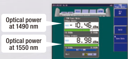
PON optical powermeter screen
